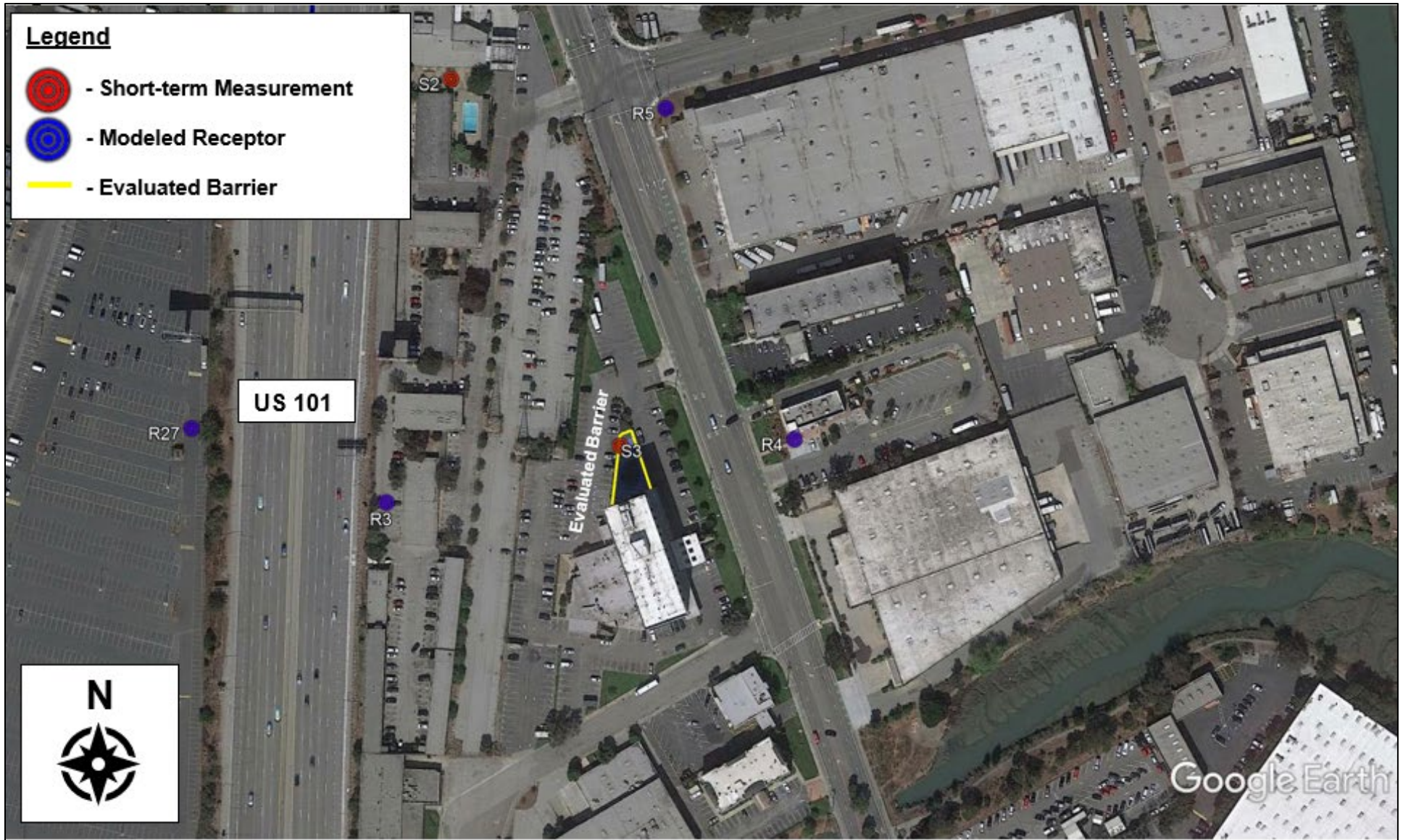
Figure 2.3.7-3 Receptor Locations and Evaluated Noise Barrier
