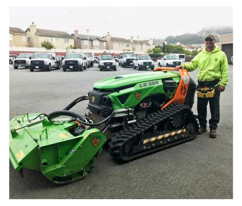
It's green, stands at more than 3-1/2 feet tall and nearly six feet wide, weighs in at 2,850 pounds, features a powerful motor that runs at 2,400 RPM, and travels at a speed of up to 5.5 mph. What is it? It's the City's Parks and Recreation Department's new remote-controlled slope mower!
