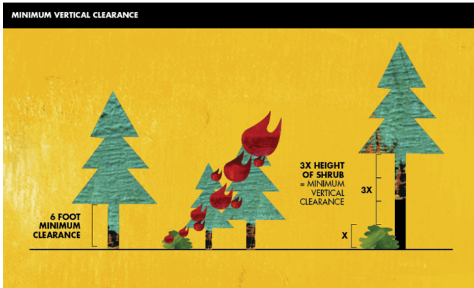
Figure 7. CAL FIRE Defensible Space Guidelines Vertical Spacing
