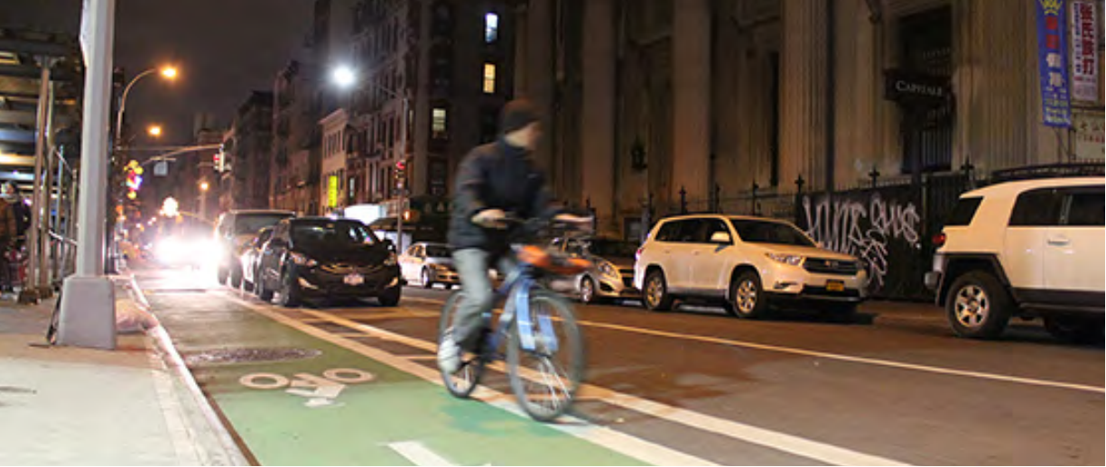
Street Level Separated Bicycle Lanes can be separated from the street with parking, planters, bollards, or other design elements.
