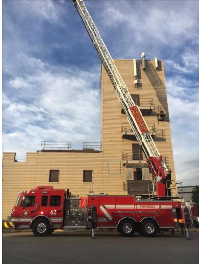
A Quint is designed to function with features of both a fire engine and an aerial ladder truck. This requires it to meet the basic needs of an aerial ladder truck, while also supplying fire hose, a water tank, and a pump. It is also outfitted with advanced communication technology to provide vital information to firefighters as they respond to incidents throughout South San Francisco.
